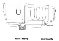
01. Install the wrist strap by snapping the triangle-shaped clip\* onto the clip holder as shown, with the clip's interior angle pointing upwards.
