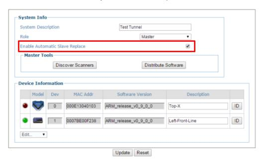
Select the **Enable Automatic Slave Replacement** check box, click **Update**, and save the system parameters as described in sections *4.8.1*, *5.2* and *5.3*.
