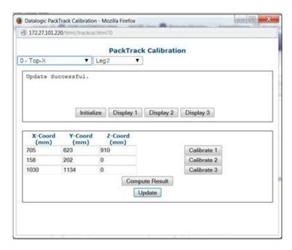
37. Close the **PackTrack Calibration Wizard** window. **PackTrack Calibration Coefficients** have been populated on the Scanner Mounting widow.
