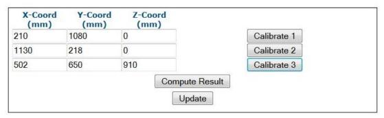
17. Click Compute Results. The results are displayed at the top of the **PackTrack Calibration** window.
