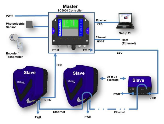
Figure 19: DX8210 Array (Tunnel) with SC5000
