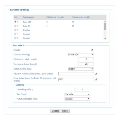
15. in **Modify Settings | Global Settings | Barcode Configuration** select single, multiple, or logical combination of labels, based on your application.
