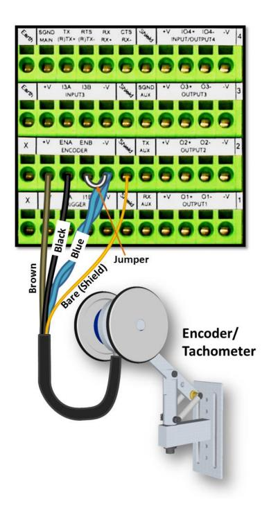
Figure 29: OEK-4 (95B082050) Encoder/Tachometer Wiring (PNP Output)
