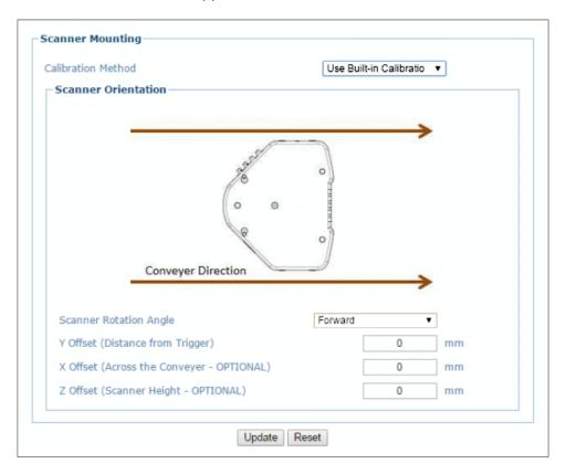
3. Select the scanners orientation to the conveyor from the **Scanner Rotation Angle** drop-down list. Selections include:
