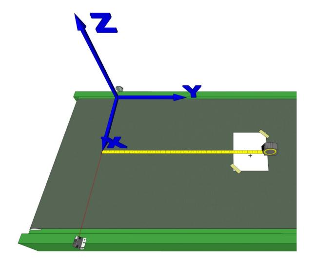
Figure 59: Measuring the Y Offset
