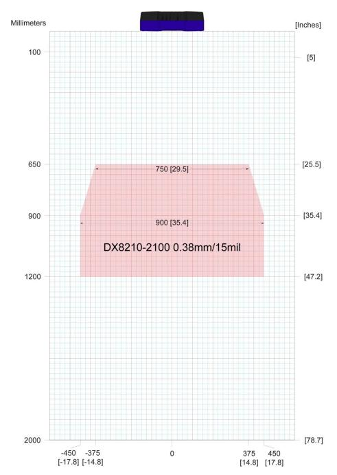
1,000 scans per second (standard) throughout DOF ANSI Contrast Grade 84% or greater ANSI "Grade A" Print Quality Pitch not greater than +/- 15  $^{\circ}$  Skew not greater than +/- 15  $^{\circ}$  Tilt not greater than +/- 45  $^{\circ}$
