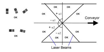
Figure 73 – X-Pattern Reading Zones with  $\alpha$  Max
