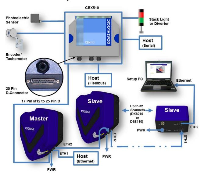
Figure 18: DX8210 Array (Tunnel) to CBX510
