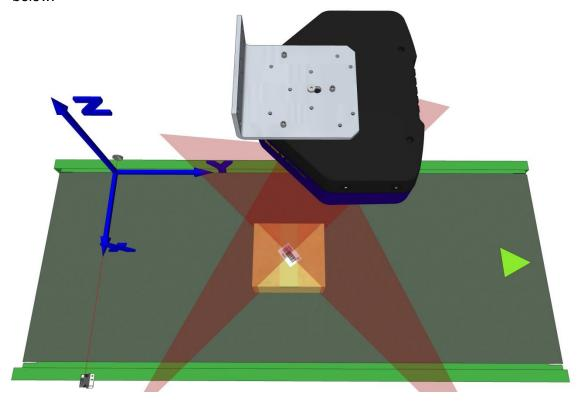
Figure 62: Test box and label placed in laser line
