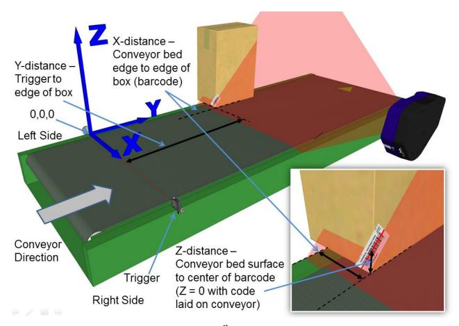
Figure 54: Side-read 1st barcode placement
