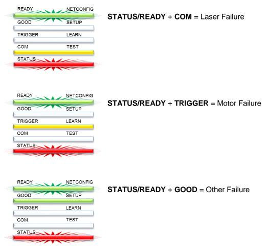
Figure 88: LED Failure Specific Indication
