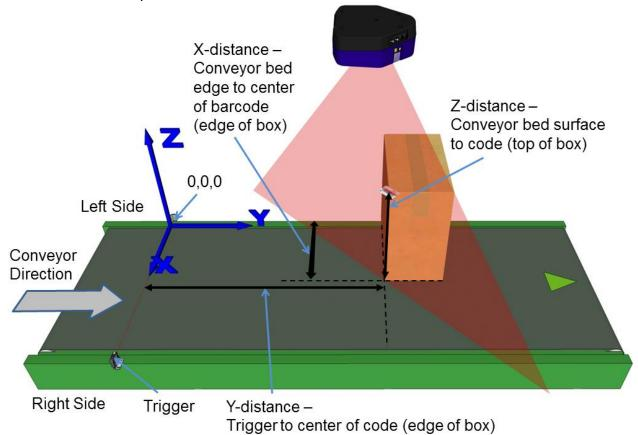
Figure 47: Top-read leg 2- 1st barcode placement
