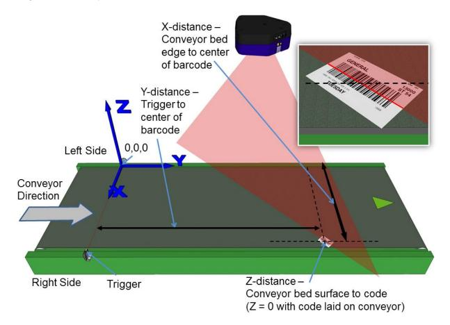
Figure 49: Top-read leg 2- 3<sup>rd</sup> barcode placement
