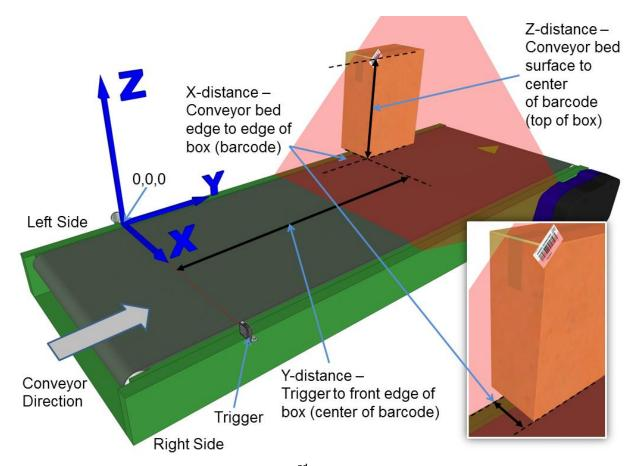
Figure 55: Side-read 2<sup>nd</sup> barcode placement
