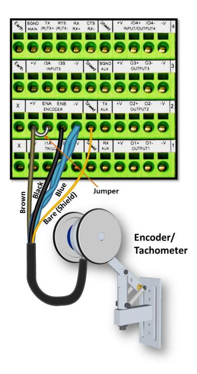
Figure 27: OEK-4 (95B082050) Encoder/Tachometer Wiring (NPN Output)
