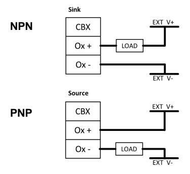
**Figure 31: Unpowered Outputs**
