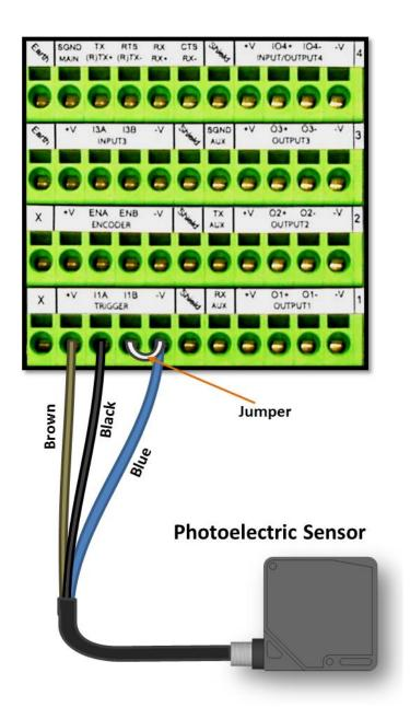
Figure 25: Photoelectric Sensor Wiring (PNP Output)
