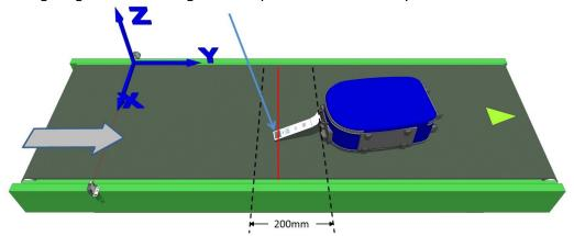
Figure 68 – Compensating for Irregular-Shaped Packages
