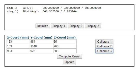
17. Click Compute Results. The results are displayed at the top of the **PackTrack Calibration** window.
