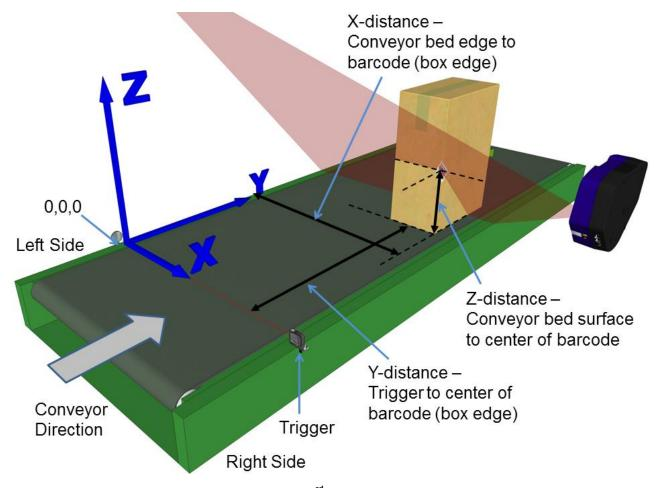
Figure 53: Side-read 3<sup>rd</sup> barcode placement
