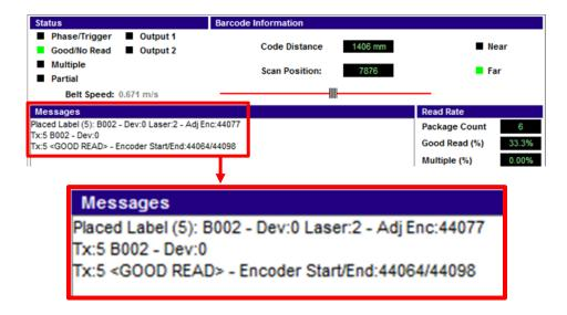
The **Adj Enc** (Adjusted Encoder) value indicates the encoder count at which the label was read. **Encoder Start/End** indicates the encoder values at the start and end of the test box.
