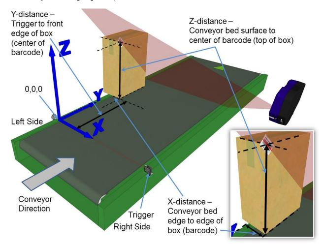
Figure 52: Side-read 2<sup>nd</sup> barcode placement
