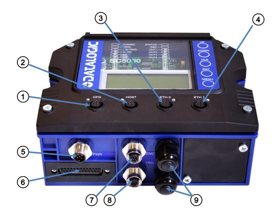
Figure 33: SC5000 Bottom Panel Connectors
