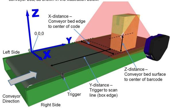
Figure 56: Side-read 3<sup>rd</sup> barcode placement
