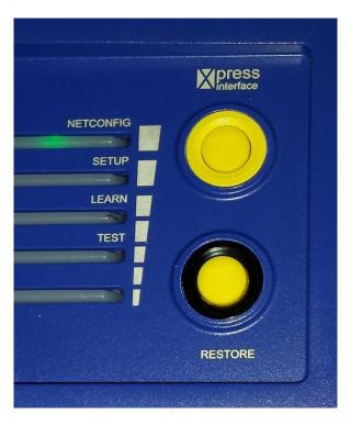
Figure 5: DX8210 X-PRESS Interface Buttons
