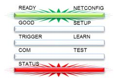
Figure 87: LED Failure Indication
