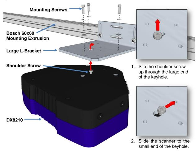
Figure 14: Keyhole mounting with large L-Bracket (Bosch 60x60 Extrusion)
