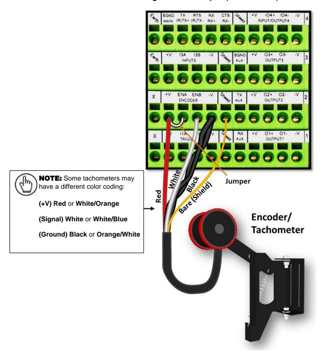
Figure 26: OEK-2 Encoder/Tachometer Wiring (NPN Output)
