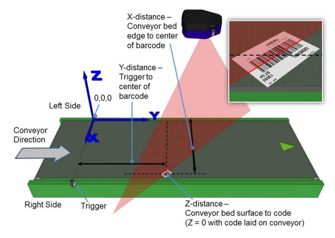
Figure 45: Top-read 2<sup>nd</sup> barcode placement
