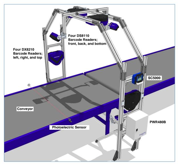
Figure 67 – Example Large Synchronized Network Reading Station
