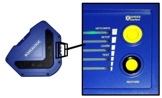
Figure 37: Control Panel Buttons
