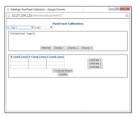
The **PackTrack Calibration Wizard** asks you to physically measure and enter barcode coordinates for the extremes of your barcode scanning system. You will measure and enter XYZ coordinates for barcodes in three different locations along each of the DX8210's laser line (legs). One leg of a **top-mounted** and **side-mounted** DX8210 scanner is shown in the illustrations below.
