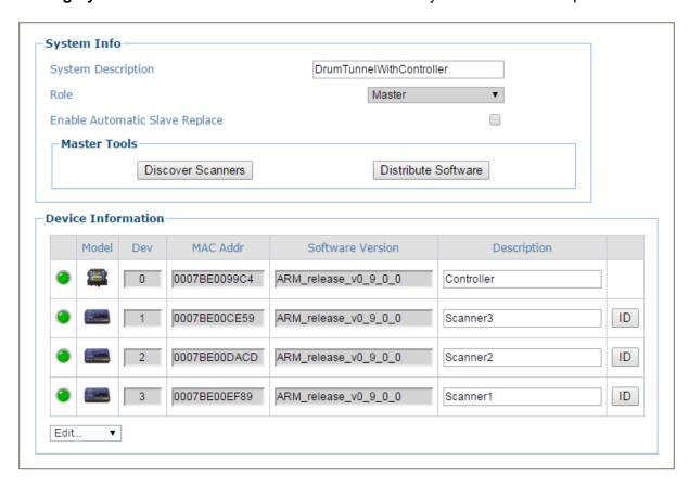
The **Device Information** section of the window should now list all of the scanners (and an SC5000 Controller if used), including the scanner you just replaced.
