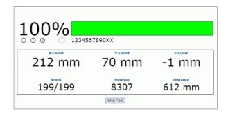
4. Physically measure the X (from left edge), Y (From PS), and Z (code height) coordinates of your test barcode, and compare your measured results to the Read Test results. Your measured results and those displayed should be close (within a few millimeters) but do not need to be exact.
