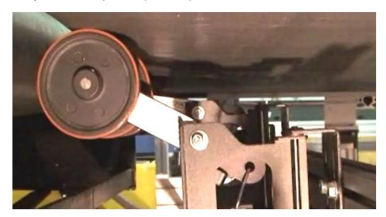
Figure 84: Tachometer Wheel
