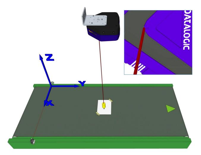
Figure 58: Using a plumb bob to mark scanner location on conveyor
