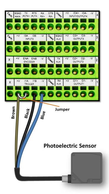
Figure 24: Photoelectric Sensor Wiring (NPN Output)
