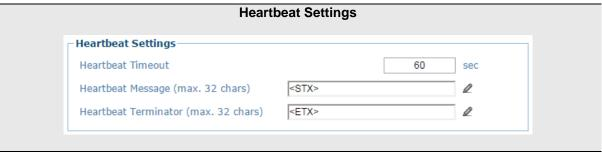
Heartbeat Timeout Enter a time value in seconds to define the amount of time between two message transmissions. If the input timeout expires and no transmission has occurred, the Heartbeat message will be transmitted.
