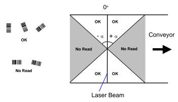
Figure 72 – Reading Zones with  $\alpha$  Max
