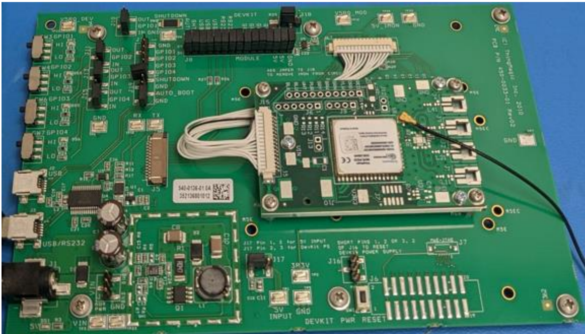
Figure 13: Carrier Board on Dev Kit Board
