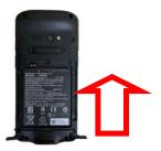
3. Lock the battery cover by turning the knobs a quarter of a turn (90°). Make sure the battery cover is securely closed, or you may be unable to turn on the terminal.
