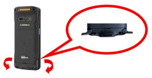
Pull the battery up to remove it.
