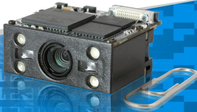
The NLS-EM3000 embedded 2D barcode scan engine, powered by advanced imaging technology and Newland patented **UIMG<sup>®</sup>** technology, a computerized image recognition system, can read barcodes on various mediums such as paper and plastic, with excellent motion tolerance.
