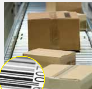
Top Side Sorting Read barcodes on fast moving ship sorter applications.
